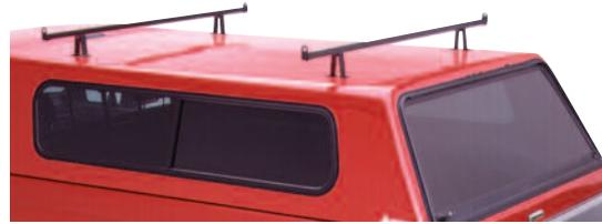
Our Load Rails are made of extruded aluminum with black electrostatic powder-coat finish. Load Rails include steel "tie downs" bolted to the ends to keep the load from sliding, and PVC inserts to help protect loads from being damaged. Mounting Legs are made of aluminum extrusion with black electrostatic powder-coat finish, and are available in three heights to accommodate the variety of camper shells on the road. Mounting Legs must be ordered separately from Load Rails.
