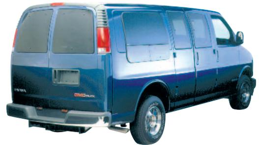
These windows combine the features, ventilation and installation ease of van conversion windows with the high-tech "aero" look of factory bonded glass. With their contoured dark solar privacy glass, silk screen frit edge, sturdy powder-coated frames, and smooth reliable hardware, CRL's "All Glass Look" Van Windows are the "cutting edge" in beauty, quality, and value!
