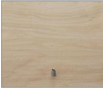
Set Fastener to Surface
