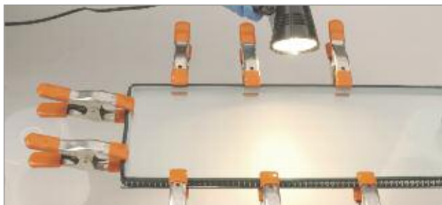
Apply Spring Clamps or Mechanical Press with Heat Lamp to seal the unit
