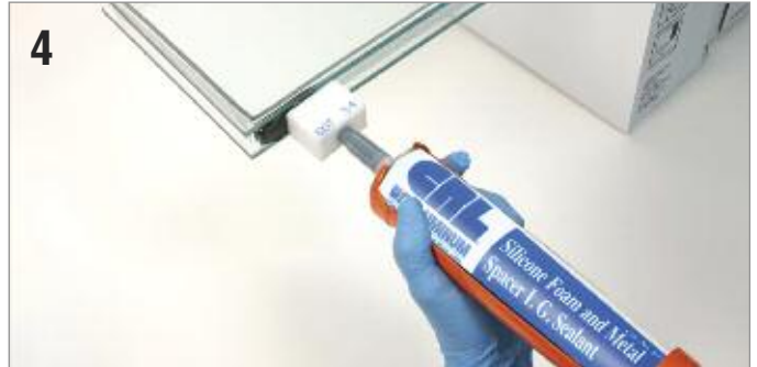
4 Apply CRL Hot Melt Butyl or Cat. No. 877 Sealant to seal the unit.
