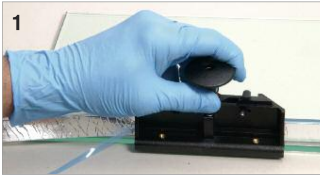
1 Apply Super Spacer® to clean glass surface with SSHN Hand Notcher or SSAPA Shuttle Applicator as release liner is removed.
