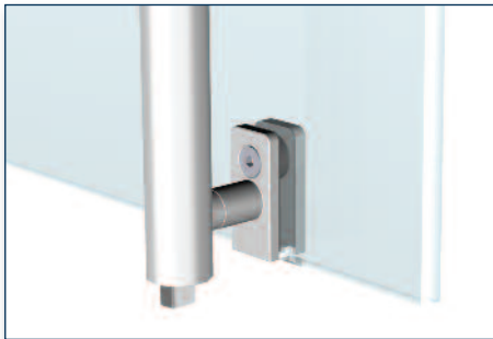
Glass Mount Detail at Latch
