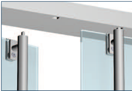
Glass Mount Detail at Latch With Header and Hole for Latch
