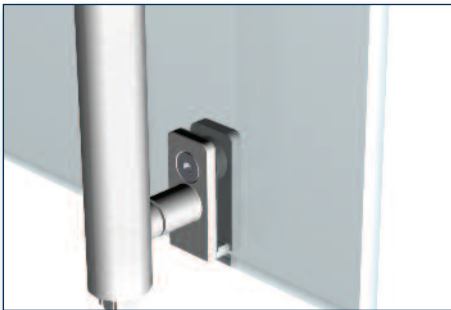
Glass Mount Detail at Latch
