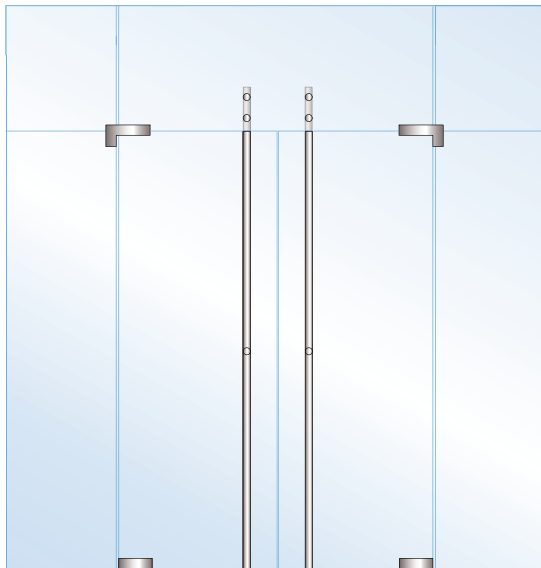
Double Door Installations Require Two Locking Handles
