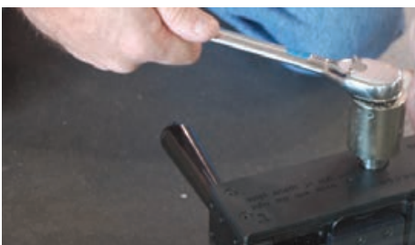
Crank the Torque Wrench until the wrench clicks and breaks for a few degrees, letting you know the Tapers are locked to the correct measured torque.
