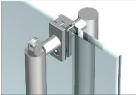
Glass Mount Detail at Latch
