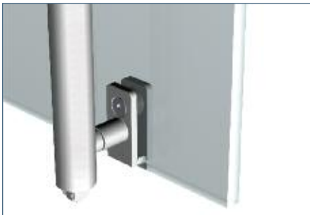
Glass Mount Detail at Latch
