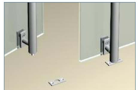
Glass Mount Detail at Latch at Floor With 777SP Flat Strike
