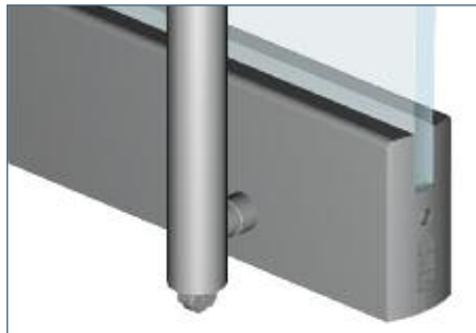
Rail Mount Detail at Latch
